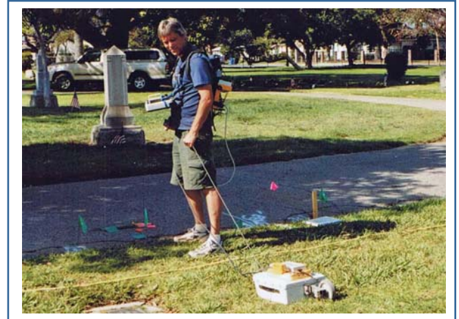
Ground Penetrating Radar in action Gary Mann of National Environmental
